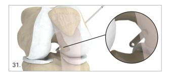
If desired, measure the length of the tunnel using the reverse length gauge (Ref. 05.05.10.0022). Insert the reverse length gauge on the distal portion of the central k-wire and slide it up to the patient bone (if necessary, make a small skin incision to facilitate instrument positioning). Evaluate the intraosseous femoral tunnel length using the distal marking of the k-wire and the scale of the length gauge.
