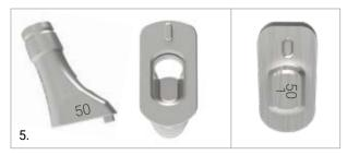
**NOTE:** Two trial necks were designed with different orientation of the pins to prevent assembly on the wrong rasps. Furthermore, trial necks compatible with the rasps 35.5 mm, 37.5 mm and 44 mm are sandblasted and the trial neck compatible with the broach 50 mm is mirror polished and bears a "50" figure etched on the base (Figure 4). The rasps have a different buttonhole orientation, as shown in the images, in order to ensure correct trial neck combination.
