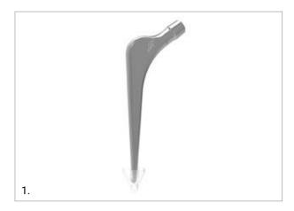
The X-acta is a highly polished, double tapered stem. This is a collarless cemented stem manufactured in wrought high nitrogen stainless steel with a PMMA distal centralizer to facilitate correct stem positioning and uniform cement distribution.
