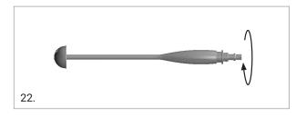
**Step 3:** Assemble the anvil and screw it until fully tightened.
