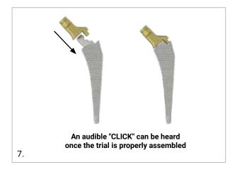
**NOTICE:** If the trial neck is not sitting well on the broach, it might be due to some lateral bone that has not been removed. Once this bone is removed, the trial neck should seat properly.
