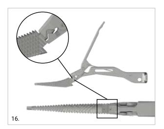
Once assembled, lower the lever and check that it is fully seated down.
