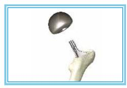
Screw the impactor adapter on the multifunction handle and use the assembly in order to perform the final impaction of the head on the stem.
