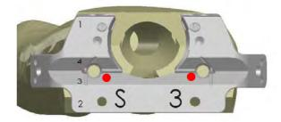
• Then pin the 4in1 cutting guide and perform the resections as described in the conventional GMK REVISION surgical technique (ref. 99.27.12US or 99.27.12).
