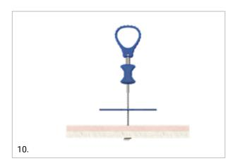
Press the counterplate towards the skin while pulling the ring handle with the other hand in order to compress and raise the soft tissues.
