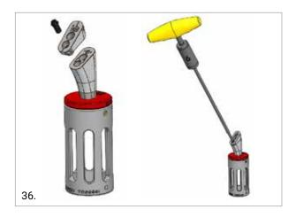
Insert the double eccenter screw into the double eccenter. Slide the M8 fixation screw into the double eccenter positioner. Screw the double eccenter onto the instrument inserting the pins into the dedicated holes.
