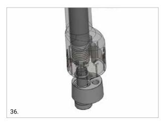
Place the double eccenter on the stem and align the markings (letters) of the instrument in the previously defined position, using the lateral line of the stem as a reference. Slide the torque limiting screwdriver T20 6 N·m into the double eccenter positioner and tighten the double eccenter screw.
